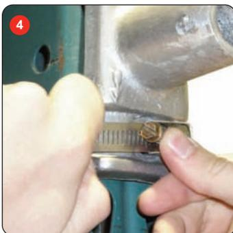
Push the screw down on the hose clamp to fasten it.
