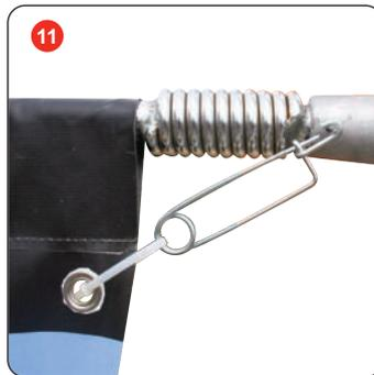
11 Use the other safety pin and fasten it to the zip tie and the safety pin holding the mount to the pole. This will make sure the graphic doesn't slide off.
