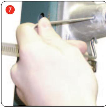
7 Push the safety pin through both holes to secure the pole in the pole mount.
