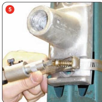
Tighten the hose clamp by turning the screw. Repeat step 2-5 for the remaining hose clamps
