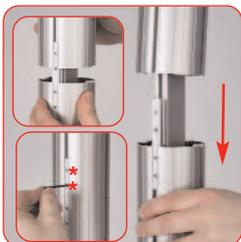
Align and slide female post over male post, tighten both grub screws using a 2mm allen key.
