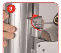
Once in position, tighten the bracket onto the linear post
