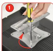
To attach the screen, align screw fixings with holes on rear of LCD screen. Fix LCD bracket in place with screws provided.
