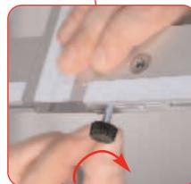
Attach adjustable foot to bottom horizontal rail.
