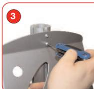
Tighten into position with an Allen Key.
